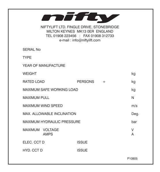
This manufacturer's plate is attached to Boom 1 on each machine at the time of manufacture on every Niftylift. Please ensure all sections have been stamped and are legible.
